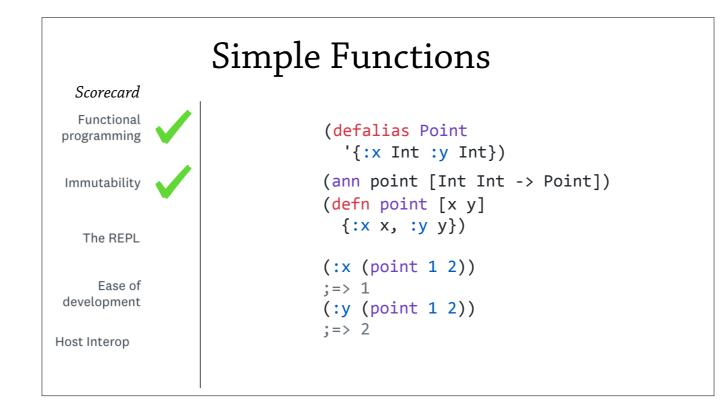
First, simple functions. Here, a function `point` is defined that takes a pair of coordinates and returns a record with two fields, x and y. On the last two lines, you can see how to lookup these fields. In fact, the curly brace syntax introduces a plain map, we are just using it heterogeneously. So to check this in TC, we add a type alias for this ad-hoc record, and annotate the function. This demonstrates support for FP and immutable data structures, since maps are immutable in Clojure.
