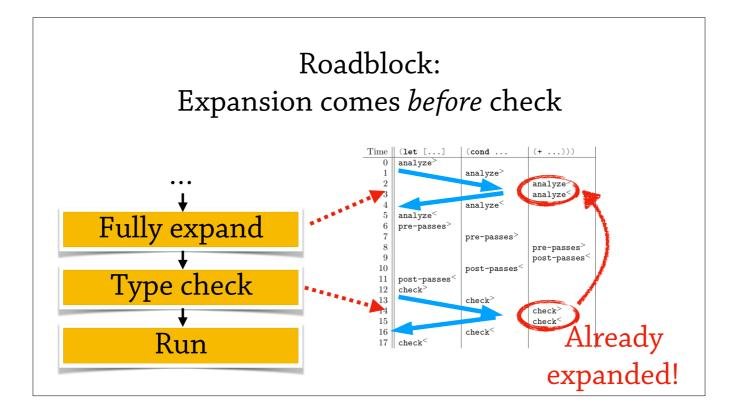
However, there's a problem. Typed Clojure fully expands code before it type checks. If we view expansion and checking as several passes over the same expression, then by the time the checker finds the expression, is has already been expanded. This is inherited from Typed Racket's design.
