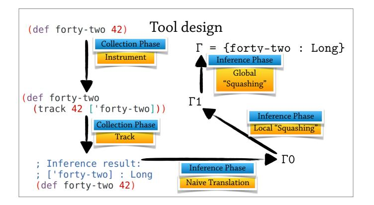
The tool is based on dynamic analysis, so it observes your running program. It's split into two phases. First the collection phase collects runtime samples, then the inference phase translates samples into an annotation. For example, to annotate this program, it is first instrumented, then tracked, and several passes are used to make compact annotations. Local squashing creates recursive types from directly nested types. Global squashing combines types from different functions.
