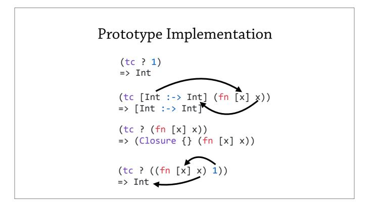
I also provide a prototype implementation for experimentation. The tc operator takes an expected type and an expression, and return the type of the expression. Integers can synthesize their type. Providing an expected type to a function triggers the usual bidirectional propagation. Omitting a type gives a symbolic closure. Applying a symbolic closure uses symbolic execution to derive the result type.
