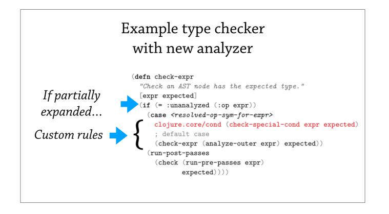
But, once this analyzer was built, we can build type checkers that interleave expansion and checking. Here's an example, where the type checker asks if an expression is partially expanded and then rules custom rules based on that.
