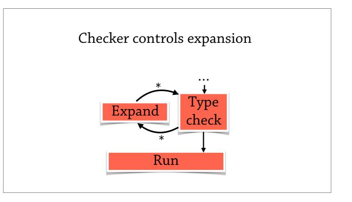
Interleaving macroexpansion and type checking, essentially gives the type checker the control over expansion. Once the checker finds an expression it knows how to check, it can fire a rule to check it.
