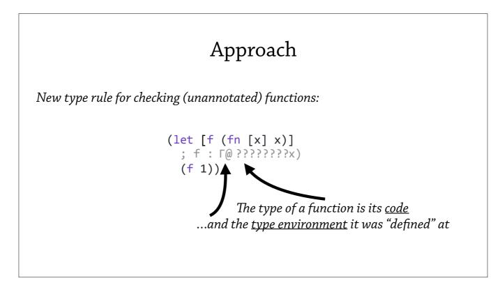
The way this is achieved is by adding a new type rule for checking unannotated functions. The type of these functions is its code, coupled with the type environment it was defined with.
