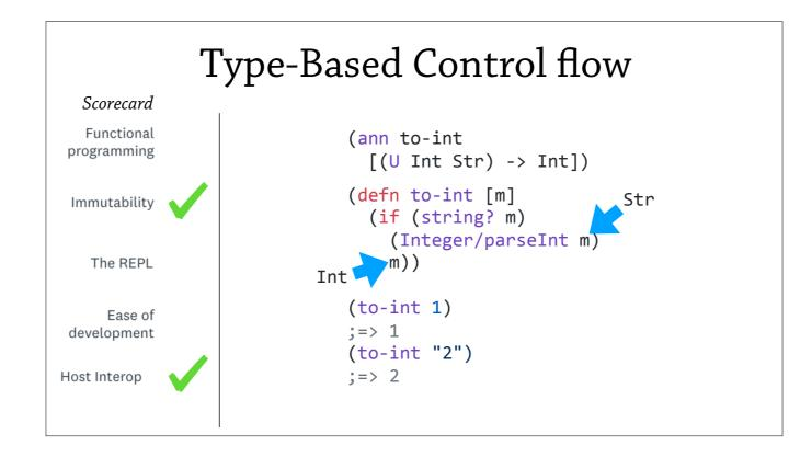
Next, an important idiom in Clojure is type-based control flow. Here, we choose branches based on the type of "m". In the then branch, we use Java interop to convert strings to ints. A union type in the annotation is all we need to check this — occurrence typing automatically follows the control flow since local bindings are immutable.
