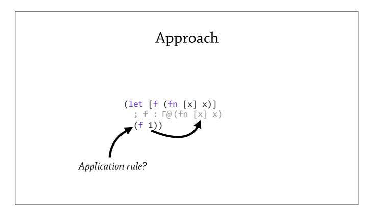
What about an application rule? The idea is that all the information to check a symbolic closure is maintained in the symbolic closure itself, and only the argument type is needed. So, we rearrange the various pieces to derive the output type.
