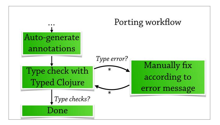
This tool is the first part of a porting workflow. First, you run the tool to generate types. Then you type check the result in TC and keep fixing type errors until it checks. The idea is that TC is a sound system so this way you get meaningful specifications in the end.
