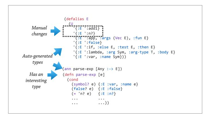
Our tool can also generate recursive types. Here's the function we're generating types for. This function creates an AST from Clojure data, and the automatically generated type is recursive and shared amongst several function annotations. However, it's missing cases due to spotty tests, and I manually had to add some cases (but only in one place).
